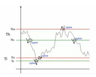
When target values are rising and exceed the positive thesholds, the device sends an uplink with the the latest measure.
